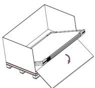
2. **Cutting packing straps**—Cutting all the packing tapes on the carton except no.1 strap and no.2 strap.
