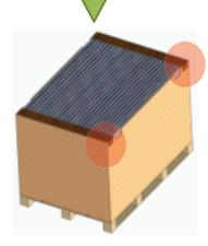
Remove the first module labeled "1" from the opening position (marked in red) firstly.
