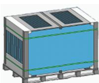
Take off the carton body vertically, and then cut off the two packing belts on top and bottom of the carton body, remove the four protecting ridges.
