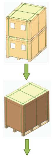
Cut off the whole packing EVA card slot on the top to belt of the pallet, and use ensure that the remaining a forklift to separate the modules are still in a fixed two pallet modules. state, and then take out all
